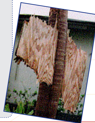
Cover photo: The roof and upper floor of this home received major wind damage from Hurricane Iniki in September 1992 (Photo: FEMA) Below: Plywood spears a palm tree during hurricane Andrew in August 1992.
